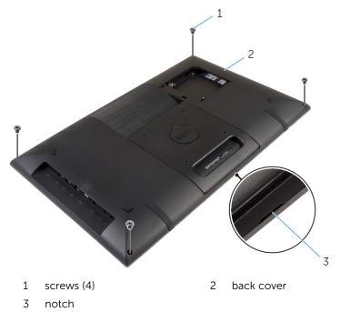
2 Using a plastic scribe, pry the back cover from the display bezel starting from the notch at the bottom of the back cover.
