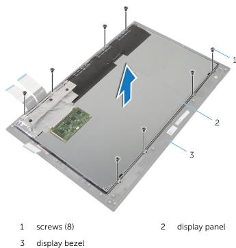
Pry the display panel off the display bezel and place it on a flat and clean surface.
